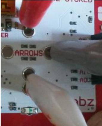
Remember, we have to connect **B** to the up arrow – red in this photo. Connect **C** to the down arrow – white in this photo and **E** to the left arrow – grey in this photo. (Don't forget, you are working on the back of the Makey Makey so left is on the 'wrong' side!).
